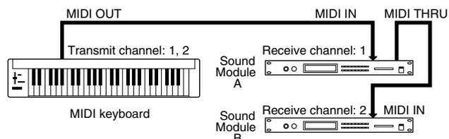
When used as a sound module, the JUNO-G can receive on up to sixteen MIDI channels. Sound modules like the JUNO-G which can receive multiple MIDI channels simultaneously to play different sounds on each channel are called multi-timbral sound modules.
