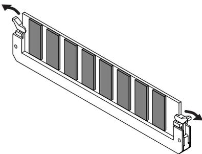
2. Remove the memory module from the socket.
