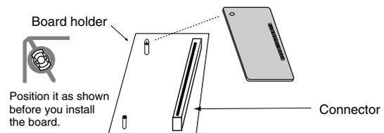
4. Use the Installation Tool supplied with the Wave Expansion Board to turn the holders in the LOCK direction, so the board will be fastened in place.
