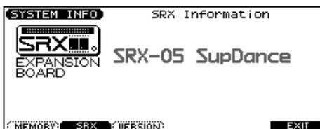
\* If the name of the board does not appear, it is possible that the board is not being recognized correctly. Turn off the power as described in **Turning Off the Power** (p. 15), and re-install the Wave Expansion Board correctly.
